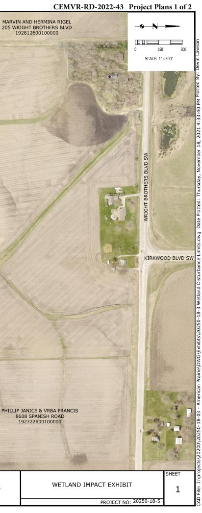
BORROW AREA FOR ROADWAY EMBANKMENT AREA=~1.00 AC CUT DEPTH=TOP 2' OF EARTHEN MATERIAL GENERATED BORROW VOLUME=~3200 CY
